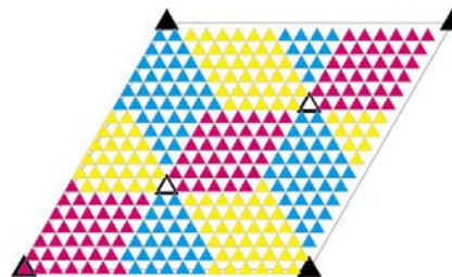
Figure 5 The FFT unit cell in the reciprocal space for N = 6 . The data points lie at the centers of the colored triangles. Red points form the chosen FFT asymmetric unit.
